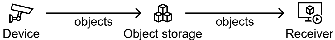
Figure B.1: Data flow for object storage recording
